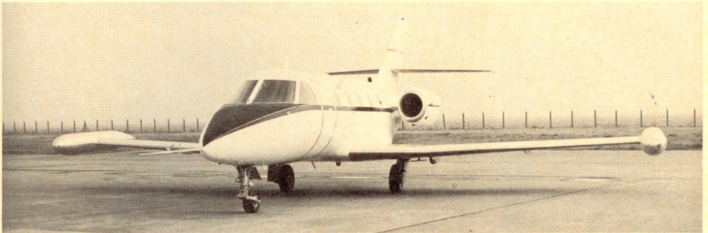
Clean and handsome, the No. 2 Corvette, with tip tanks, climbs to 20,000 feet in seven minutes. The two Pratt & Whitney (UACL) JT15D-4 turbofans combined will produce 4,620 pounds of thrust.
